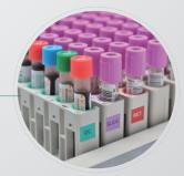
The special tube racks utilize different barcodes to differentiate specific usages, such as "QC", "Slide making & staining only" and "RET test only". The special tube racks can carry the tubes to perform these specific functions in the simplest way.
