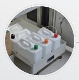
All reagents as well as the pneumatic unit can be set in the trolley below respective BC-6800 or SC-120. In this manner, the reagents and pneumatic unit are well organized permitting easy reagent replacement.
