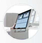
The touch screen is the "brain" of CAL 8000. It optimizes the distribution of workload between each BC-6800 unit and decides which sample requires a blood smear. It displays the status of each BC-6800 or SC-120 installed on CAL 8000 as well as the volume of balance reagent. This intuitive software can tell the users all necessary information of CAL 8000 at any given time. Consequently, the users will spend less time operating CAL 8000 and arrange their working schedule better.
