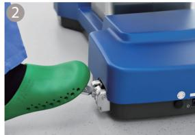
Step 1: Turn the knob clockwise to enter the Manual Override System mode.
