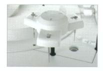
Effective mixer unit Independent mixing units for reagents and samples. Threehead mixing bars improve performance. Two-grade washing reduces contaminants significantly
